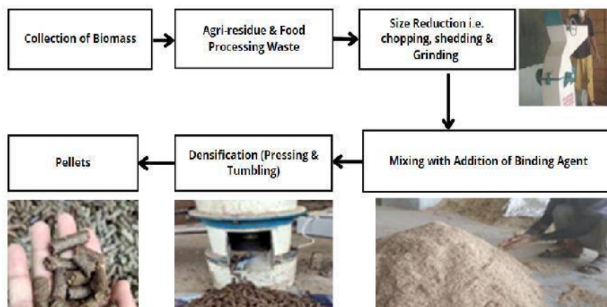
Figure 2: Process flow of pelletization
