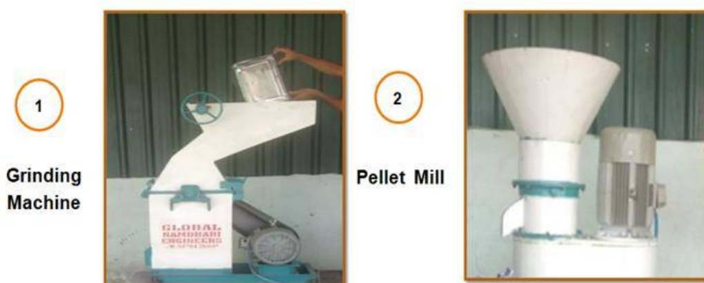
Figure 1: Pictorial view of pilot pelletization unit used for experimentation
